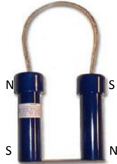
Natural Magnet Test: 9.8 kg lift each
