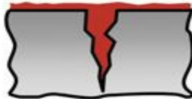
3 Application of penetrant
