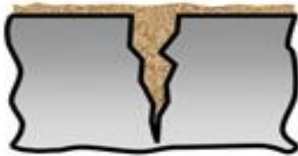
1 Crack filled with dirt
