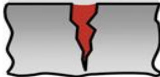
5 Application of developer
