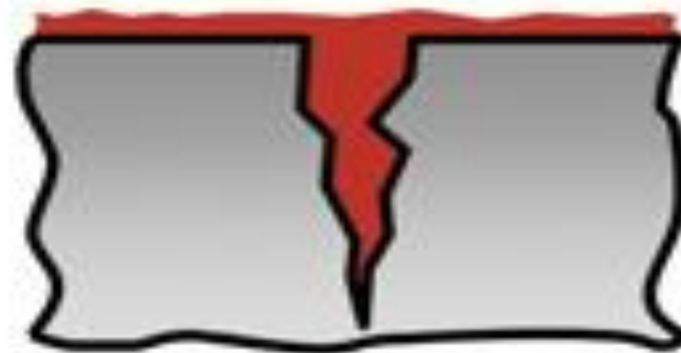
3 Application of penetrant
