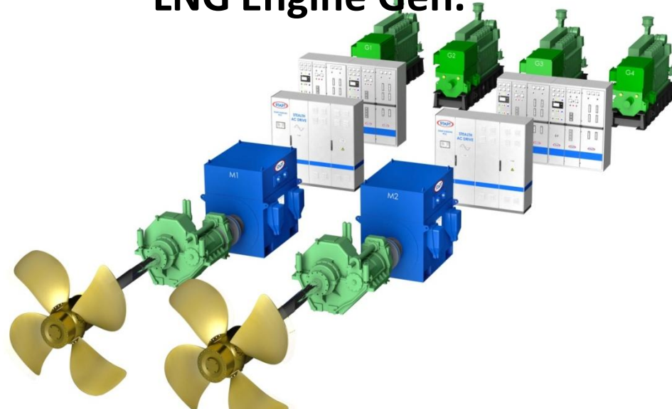
Engine Room, Elc.Motor Propulsion system
