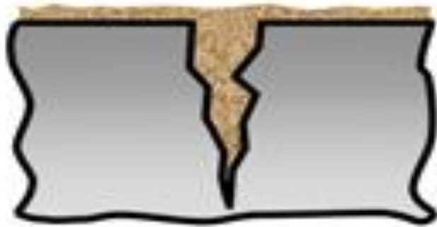
1 Crack filled with dirt
